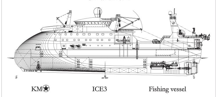
TRAWLER 87m big freezing processing trawler with a possibility of fish catching with bottom and pelagic trawl, designed for maximum fishing efficiency. The design based on the well-established and proven Enduro TM Bow concept for the best seaworthiness in rough seas. This bow shape also allows full use of the vessel for the benefit of the crew and the maximum capacity of the fish hold and the vessel as a whole.
