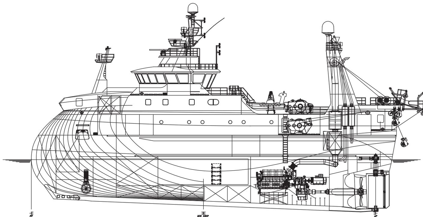
КМ★ ICE2 (hull) ICE1 (machinery) AUT1 Fishing vessel
