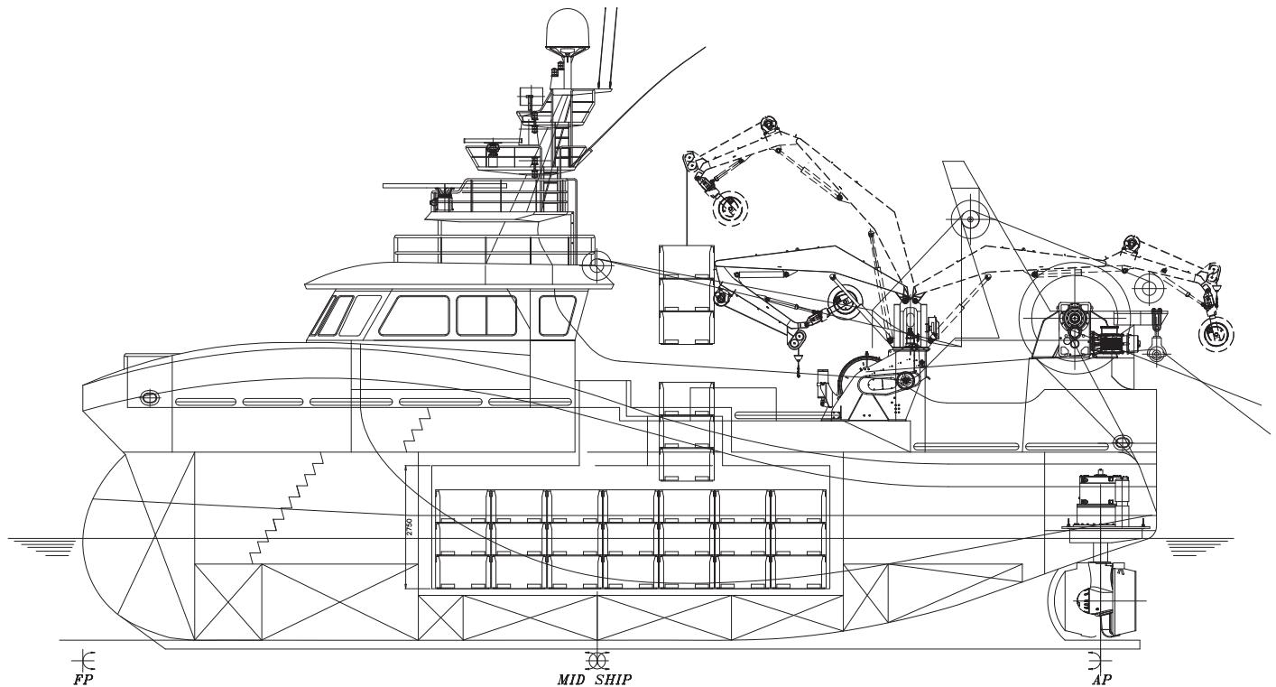
**KM★ ICE2 (hull) ICE1 (machinery) R2 - RSN AUT1 Fishing vessel**
