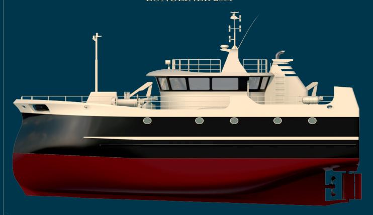
KM ICE2(hull) ICE1(machinery) R2 - RSN AUT 1 Fishing vessel
